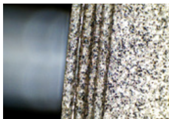
D64 wheel with small grooves
